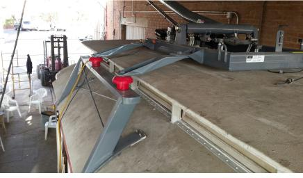
Photo on the left shows the mounting system designed by OPT members Chuck Krause and Skip Moen for the Lisbon car's new pantograph which matches those used on Tucson's modern streetcar.
