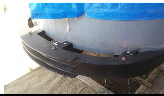
The car's bumper was modified with an imposing anti-climber which keeps one car from riding up on another in the case of a collision.
